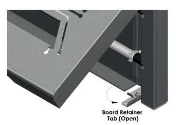
Figure 2 – Board Retainer Tabs
