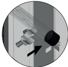
Figure 3. Removing the lamp from metal support clip.
